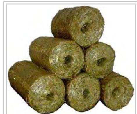
Biomass briquettes are an example fuel for production of dendrothermal energy
