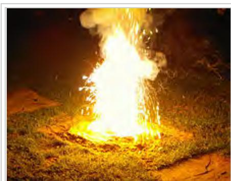
A thermite reaction using iron(III) oxide
