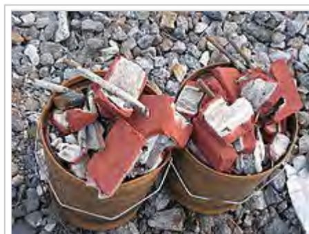
Residues of ceramic molds for thermite welding like these, left by railway workers, can be found along tracks
