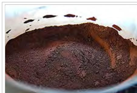
A thermite mixture using iron (III) oxide
