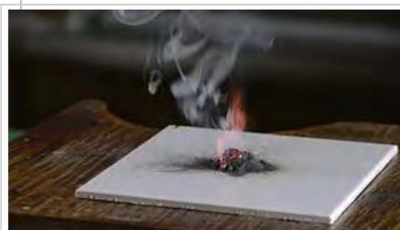
Demonstration of the reaction between a strong oxidising and a reducing agent. When few drops of glycerol (reducing agent) are added to powdered potassium permanganate (strong oxidising agent), a vigorous reaction accompanied by self-ignition starts.
