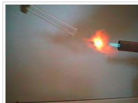
Match test used to detect the presence of hydrogen gas
