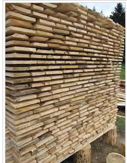
Air-drying timber stack
