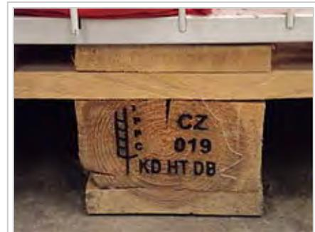
These IPPC markings on a wood pallet indicate KD: kiln-dried, HT: heat treated, and DB: debarked. Essentially all wood packaging material that is exported to an IPPC member state must have a stamp such as this.
