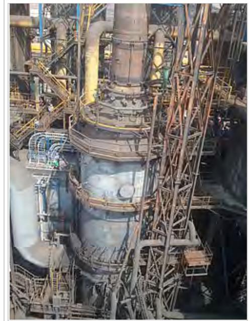
Part of the gas cleaning system of a blast furnace in Monclova, Mexico. This one is about to be de-commissioned and replaced.
