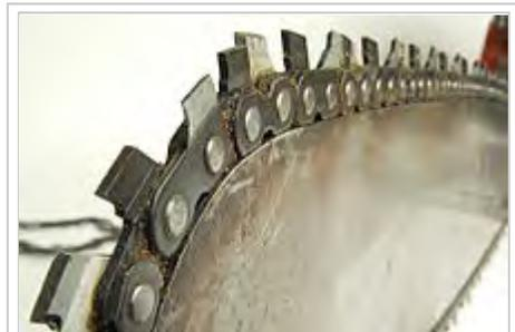
A section of "scratcher" chain on a bar nose, showing the tooth layout.
