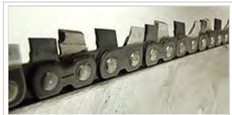
A section of "scratcher" chain showing the large number of teeth compared to modern chain.
