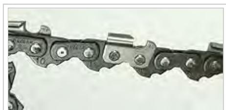
Oregon (brand) no.10 chipper chain, note the long curve between the top and side plates.
