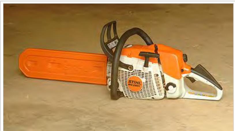
A chainsaw, with protective scabbard over the bar and chain
