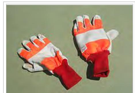
Chainsaw gloves. Note that only the back of the left hand glove contains chainsaw protective fabric, and so only that glove carries the chainsaw label.
