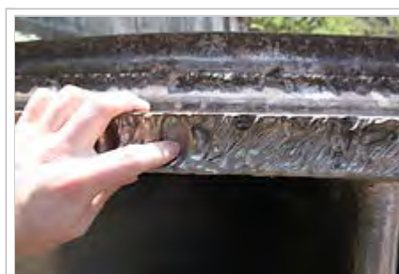
Water turbine from the Agoyan Hydroelectric plant eroded by volcanic ash laden water.
