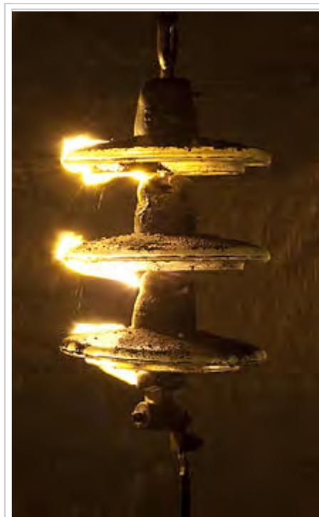
Electrical insulator flashover caused by volcanic ash contamination.
