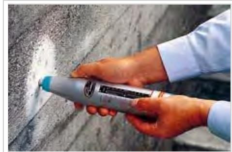
Original Schmidt Concrete Test Hammer
