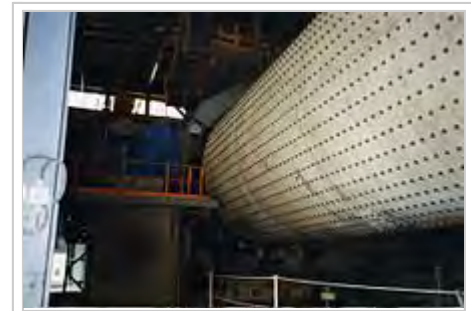
A 10 MW cement mill, producing cement at 270 tonnes per hour
