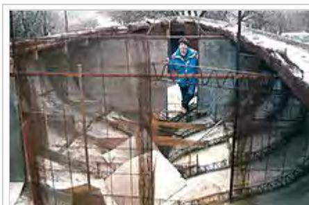
Ferrocement hull under construction
