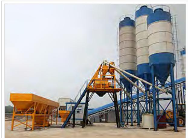
Different with the belt conveyor concrete plant, hopper "skip hoist" lift concrete plant transport aggregates to the mixer by a hopper, which is a slower way of transporting aggregate.
