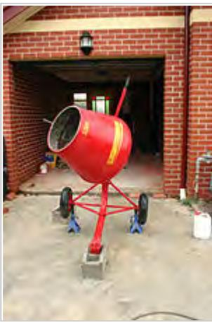
This portable concrete/mortar mixer has wheels and a towing tongue so that it can be towed by a motor vehicle and moved around the worksite by hand, and its rotation is powered by mains electricity. The lever allows the concrete/mortar to be tipped into a wheelbarrow.
