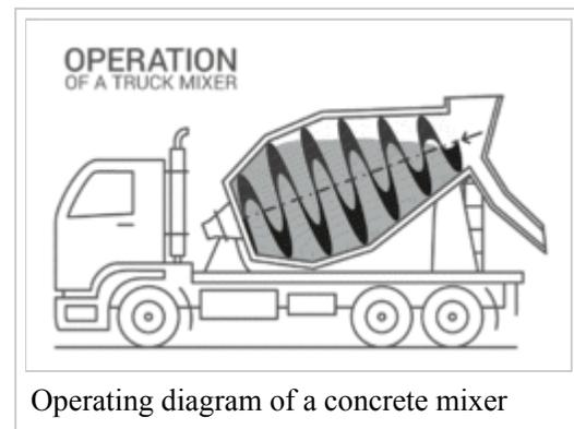
Operating diagram of a concrete mixer
