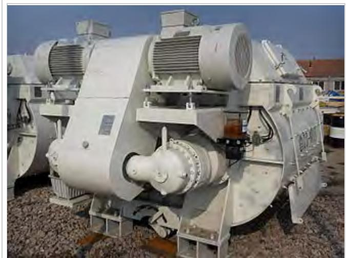
Twin shaft concrete mixer for concrete plant
