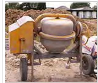
An outdated model of a small-scale concrete mixer. These older mixers are heavy and can not be moved as easily. They are still self powered with an electric motor.
