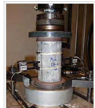
Compression testing of a concrete cylinder
