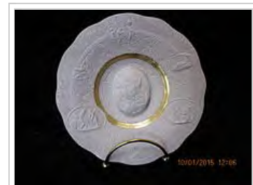
Decorative plate made of Nano concrete with High-Energy Mixing (HEM)
