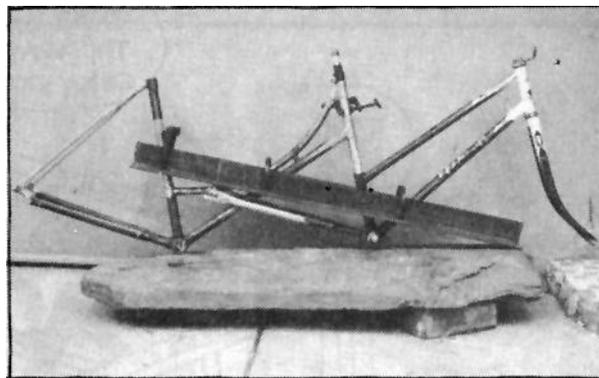
weld. (If stays are long enough weld onto curved top tube as well for extra strength).
