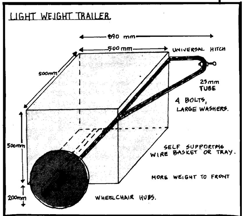
Heavy trailers must have ball joint universal hitches due to high impulse loads and tension. The rod ends from automobile steering systems are good (and cheap). To prevent the bike frame (and rider) being twisted on overturning a laden trailer, it is good practise to enable the joint to rotate under high stresses.
