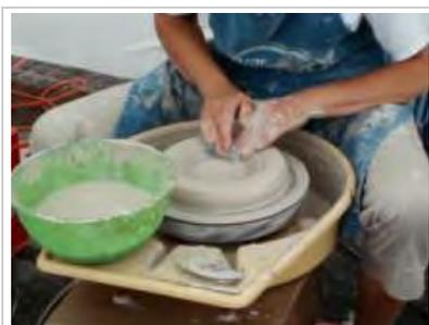
A potter shapes a piece of pottery on an electric-powered potter's wheel
