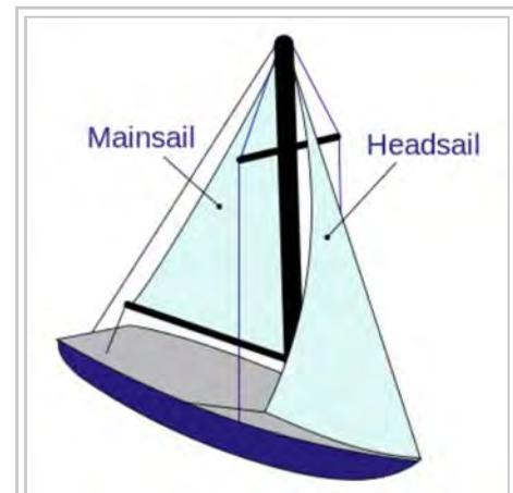
Diagram of a Bermuda or Marconi rig on a typical monohull sloop
