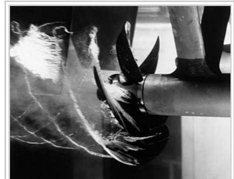
Cavitating propeller in water tunnel experiment
