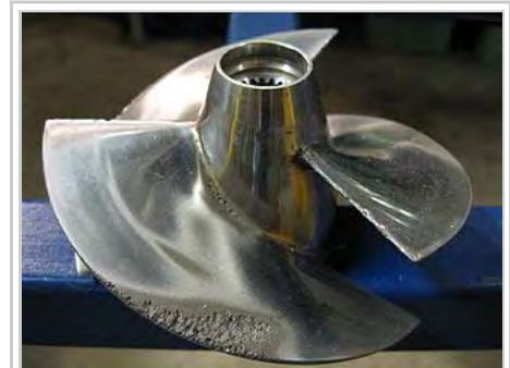
Cavitation damage evident on the propeller of a personal watercraft.
