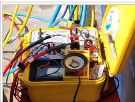
A hard-wired diver communications unit mounted in a waterproof box for convenience of transport and protection. The loose speaker has been added to increase output volume. there is a built in speaker behind the perforations on the panel.
