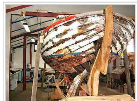
Damaged boat mid-reconstruction; carvel planking partially removed.
