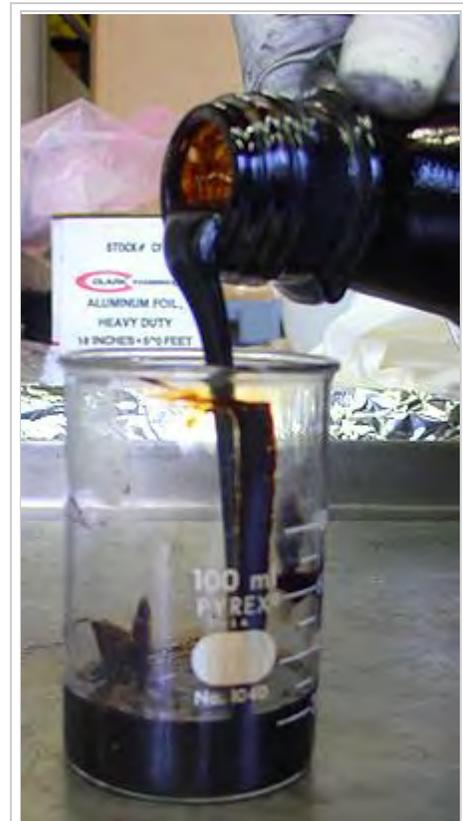
A tar-like substance can be produced from corn stalks by heating in a microwave. This process is known as pyrolysis.
