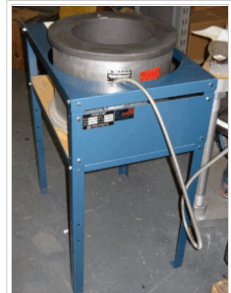
An electric melting furnace
