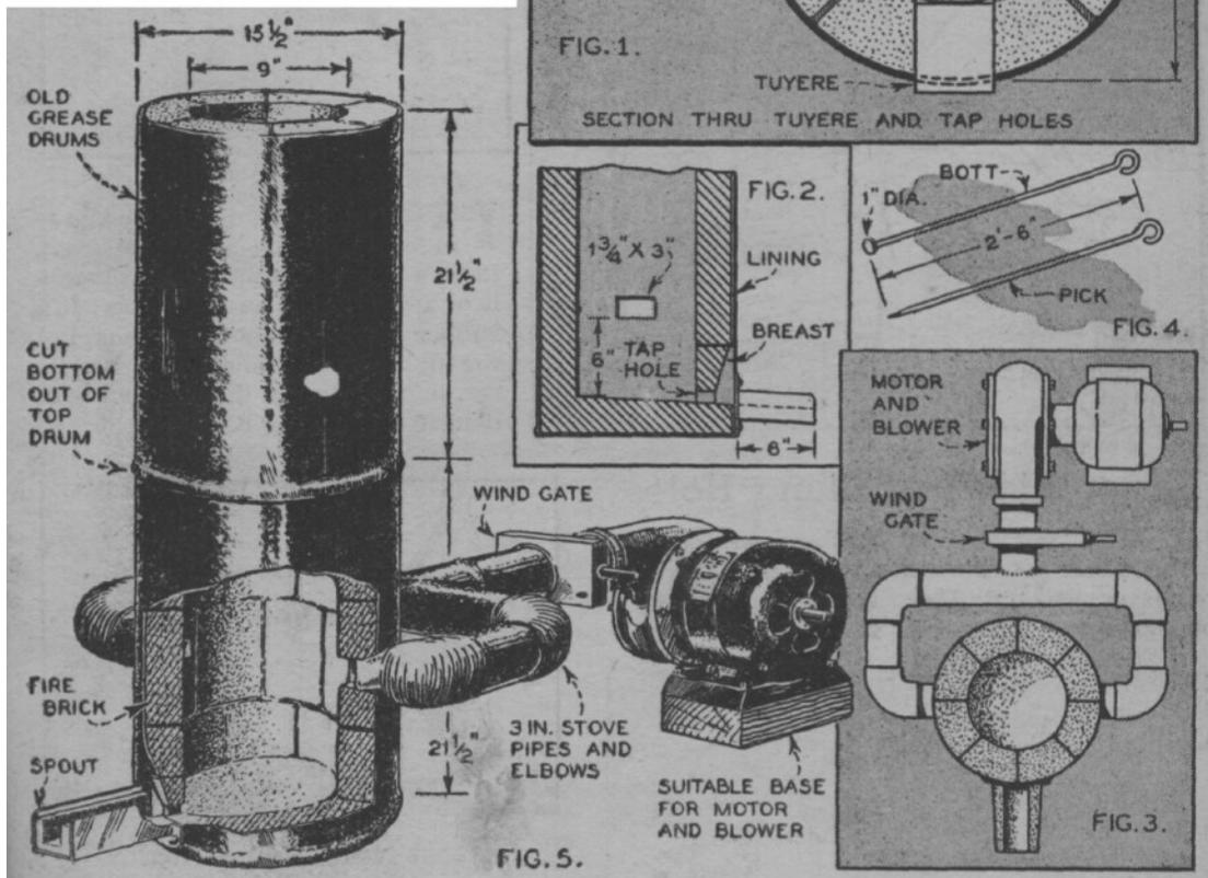
here, a line going to each tuyere. The piping is 3-inch stove pipe with the necessary ells. The windgate can be made up for you by a tinner. It is a simple sheet metal box with a movable slide to regulate the opening, and thus the air supply. Stove pipe makes an inexpensive and easily renewable air line. However, if a more permanent system is desired, 3-inch gas pipe may be used.
