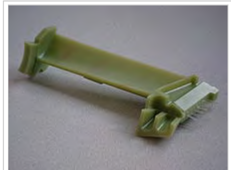
A wax pattern used to create a jet engine turbine blade
