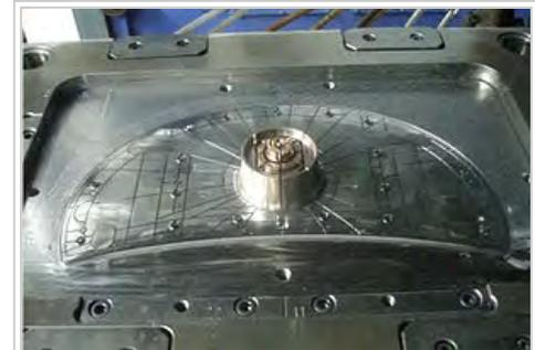
Beryllium-copper insert (yellow) on injection moulding mould for ABS resin
