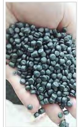
Thermoplastic resin pellets for injection moulding
