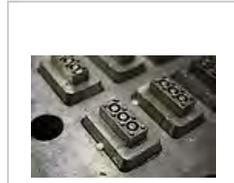
Lego injection mould, detail of lower side
