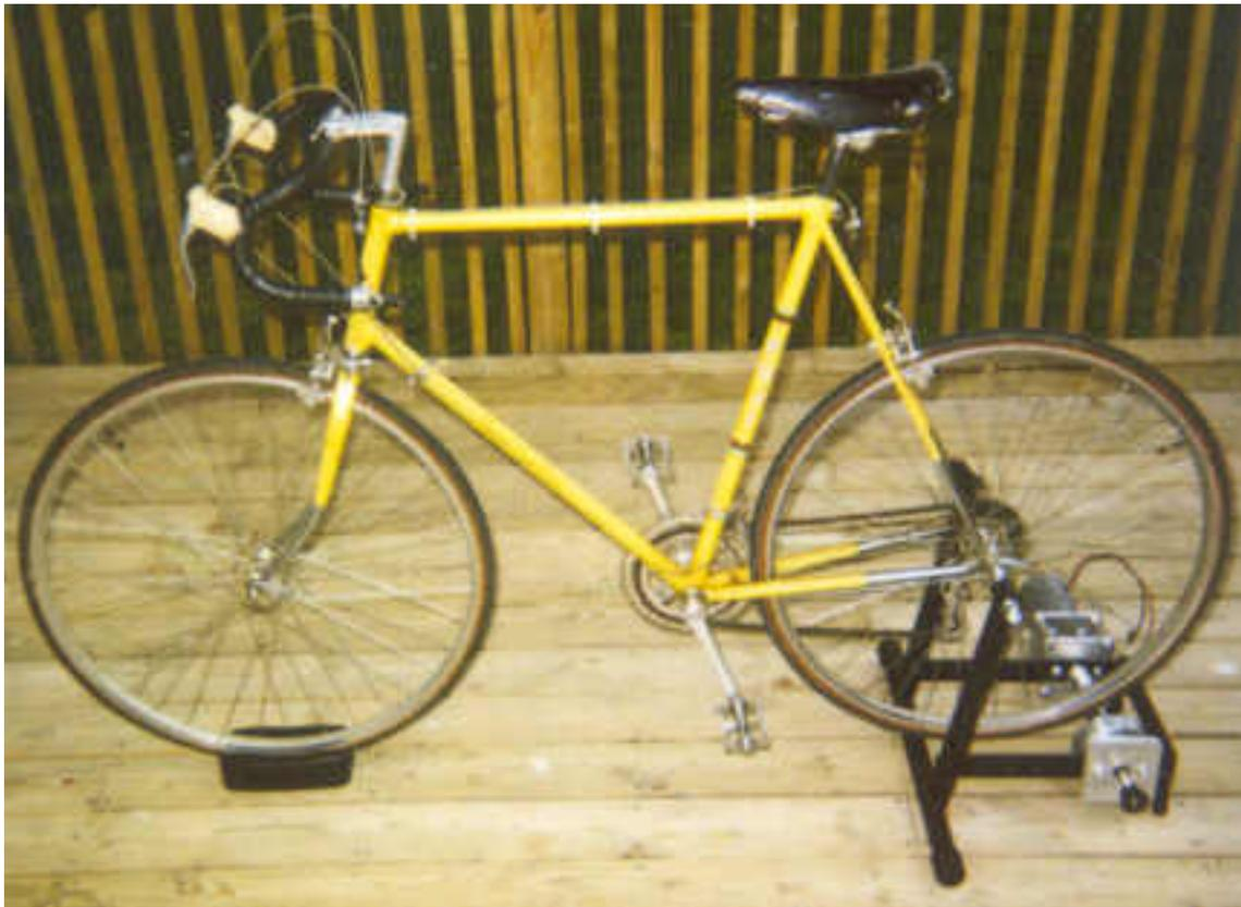
To make a long story short I bought the most versatile training stand I could find and then did extensive modifications to the roller assembly. Originally the ball bearings were pressed into the bore of the roller at the outer ends. The roller assembly spun on a stationary axle fixed to the frame. The end of the roller, opposite the integral three pound flywheel, drove the hub of a centrifugal clutch. The shoes of the clutch engaged a stationary drum which provided resistance
