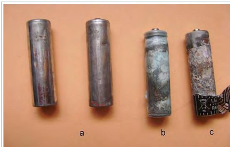
Progressive corrosion of zinc–carbon batteries.
