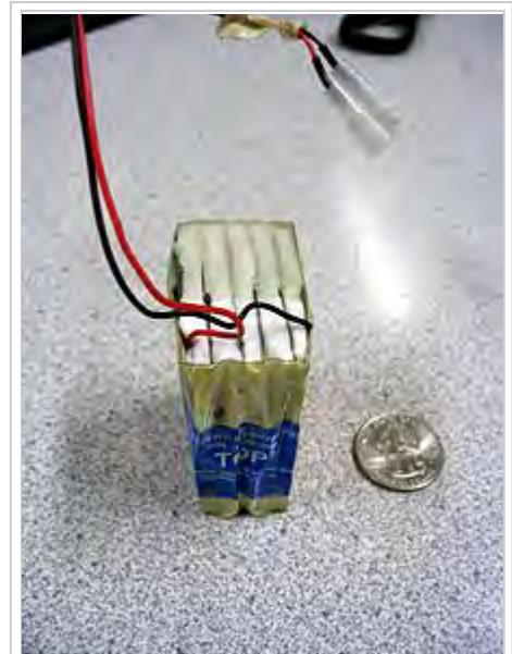
Side-view of water-activated radiosonde battery
