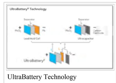
The lifetime of a battery depends on how it is used, and how many cycles of charging and discharging it is put through. In a situation where batteries are put through four 40% cycles per day and where throughput is the life-limiting factor, UltraBattery will last about three to four times longer than a conventional VRLA battery.<sup>[5]</sup>
