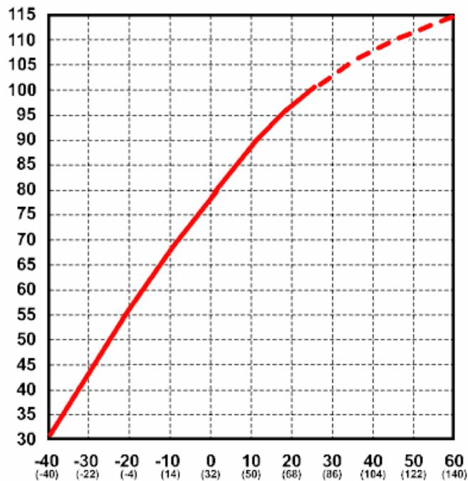
Even though battery capacity at high temperatures is higher, battery *life* is shortened. Battery capacity is reduced by 50% at -22 degrees F - but battery LIFE increases by about 60%. Battery life is reduced at higher temperatures - for every 15 degrees F over 77, battery life is cut in half. This holds true for ANY type of Lead-Acid battery, whether sealed, gelled, AGM, industrial or whatever. This is actually not as bad as it seems, as the
