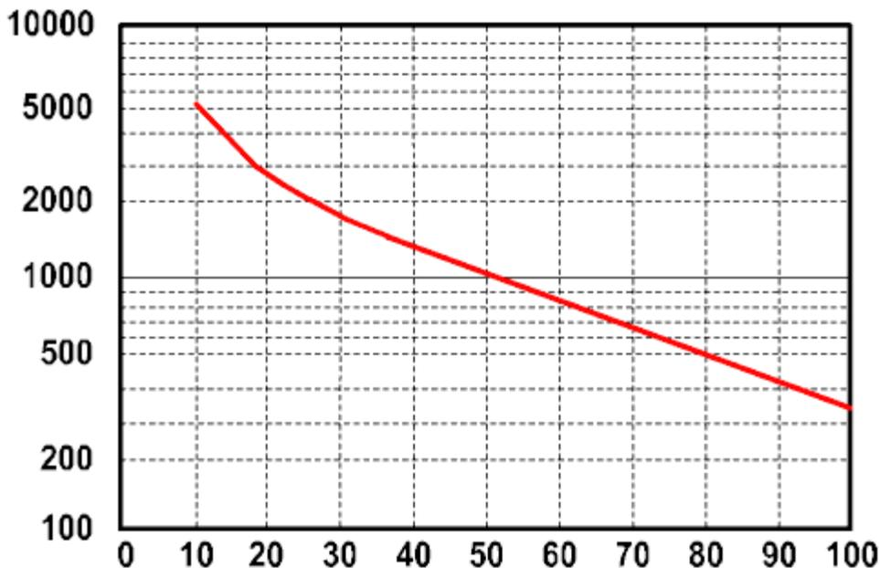
Battery life is directly related to how **deep** the battery is cycled each time. If a battery is discharged to 50% every day, it will last about twice as long as if it is cycled to 80% DOD. If cycled only 10% DOD, it will last about 5 times as long as one cycled to 50%. Obviously, there are some practical limitations on this - you don't usually want to have a
