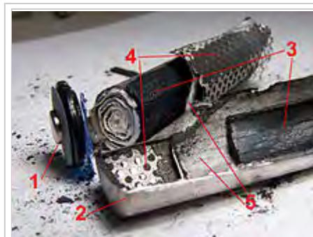
Disassembled NiMH AA battery:
