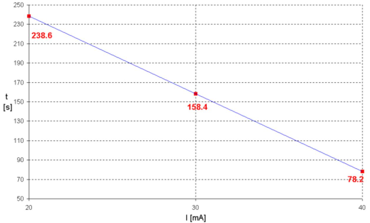
**Fig. 7: Plot of amperage versus the discharge time**
