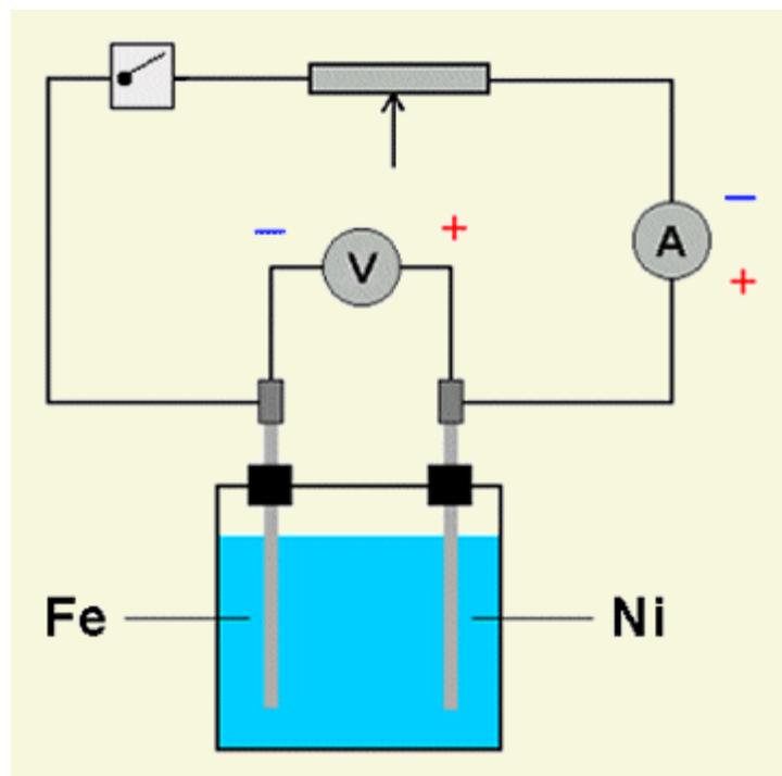
**Fig. 3: Battery discharge**
