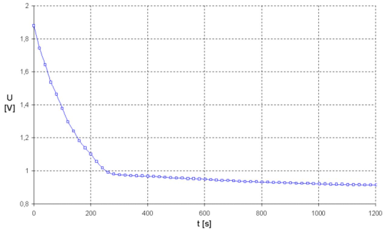
**Fig. 4: Self discharge of the Edison cell**
