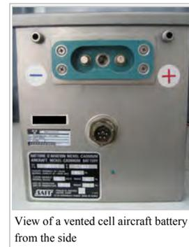
View of a vented cell aircraft battery from the side
