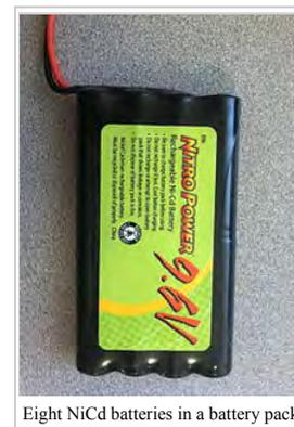
Eight NiCd batteries in a battery pack
