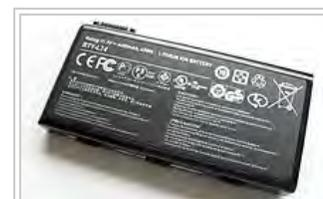
A lithium-ion battery from a laptop computer (176 kJ)
