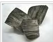
Lithium ingots with a thin layer of black nitride tarnish
