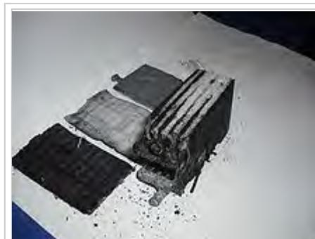
Disassembled AGM battery. From left: positive plate, glass mat separator, negative plate. On the right are the five remaining cells (of the six-cell battery).
