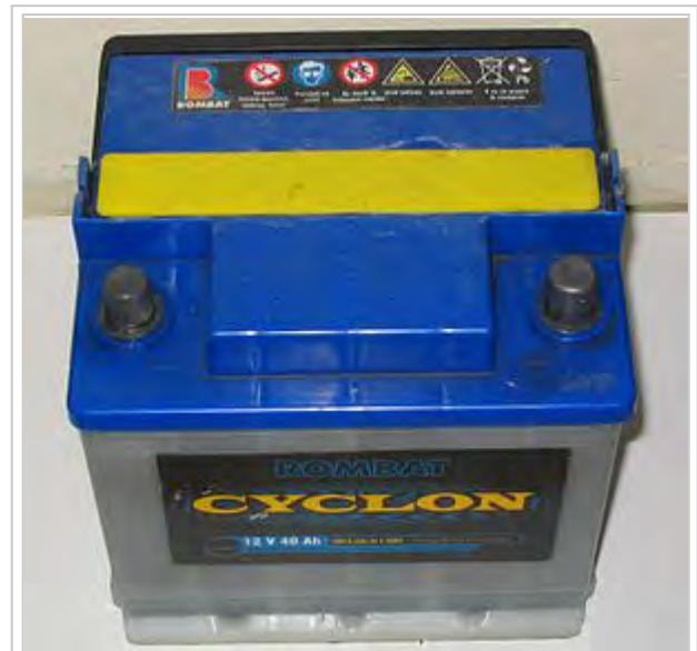
A typical 12 V, 40 Ah lead-acid car battery
