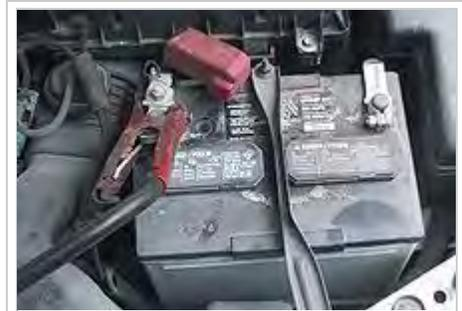
A positive (red) jumper cable connected to battery post. An optional hydrometer window is visible by the single jumper clamp. (The black negative jumper clamp is not shown.)
