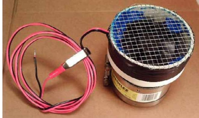
Cut a screen to keep large particles out of the fan. Tape it on with some electrical tape.
