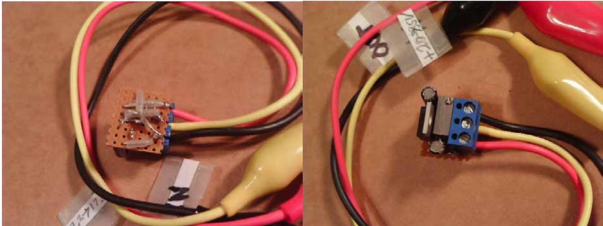
A small piece of project PC board was used. Note the adjustment 25 Turn pot in the center.
