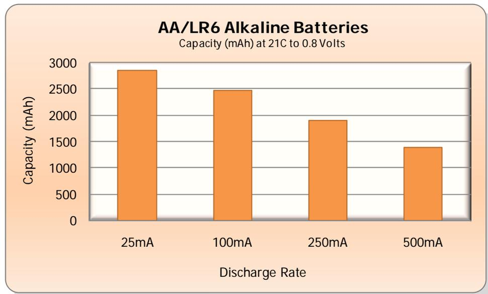
(fig. 13) AA/LR6 alkaline battery capacity to 0.8 volts
