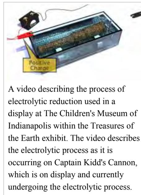
A video describing the process of electrolytic reduction used in a display at The Children's Museum of Indianapolis within the Treasures of the Earth exhibit. The video describes the electrolytic process as it is occurring on Captain Kidd's Cannon, which is on display and currently undergoing the electrolytic process.
