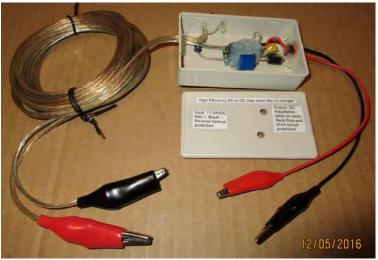
Input 11 to 24 Volts DC is on the left and the adjusted lower DC output is on the right. This unit converts input to AC then steps it down in voltage and rectifies it. It has a measured efficiency of about 80% to 90%. When conserving input power is needed this approach is much better than using a resistor or wall warts to adjust the voltage and current flow.
