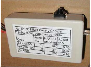
Adjust the voltage according to the table shown above. 5.86 volts or for 4AA-4AAA cells is the proper voltage for driving the two 3 watt white LEDs at about 1.1 watt. See below. The unit can be used as a USB charger (if adjusted for 4.95v) or for changing 9V NiMH or for charging 4AA or 4AAA cells or running two 3Watt LEDs in series. Put the test 390 ohm resistor across the leads as a load when adjusting the voltage.
