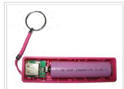
Many powerbanks use the common 18650 size lithium-ion battery which may or may not be user-replaceable.
