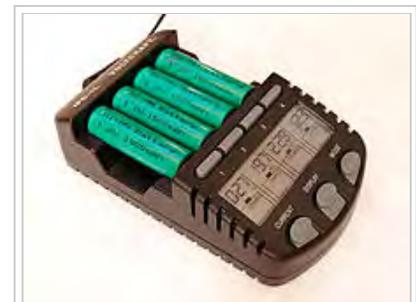
Example of a smart charger for AA and AAA batteries
