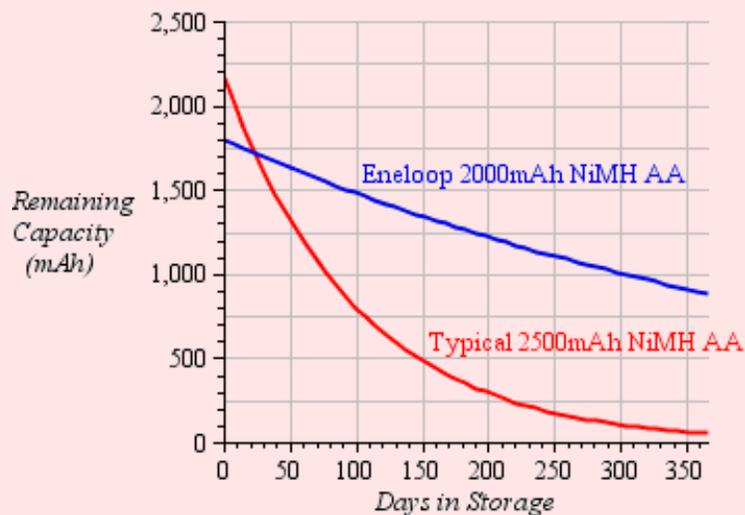
After only three weeks of storage, traditional 2500mAh NiMH cells will have less capacity remaining than 2000mAh Eneloops.
