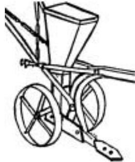
Figure 44: Ripper-planter attachment to the common plough.
