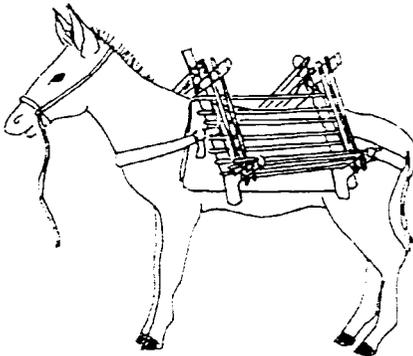
*Tie sticks with twine or fibre to make two equal four-sided boxes, one for each side of the donkey. Each side may take up to 15 bricks, depending on sizes of donkey and sticks, but load must balance evenly.*
