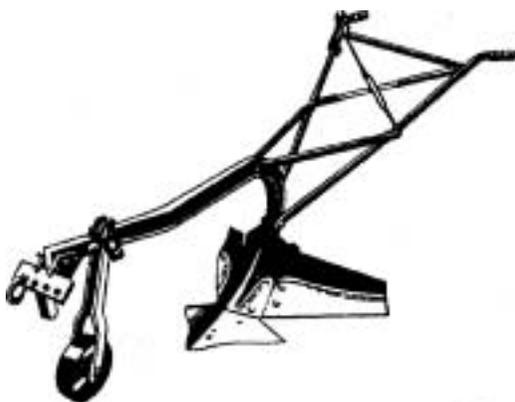
*Figure 39: "Inkunki" high wing ridger, manufactured in Zimbabwe.*
