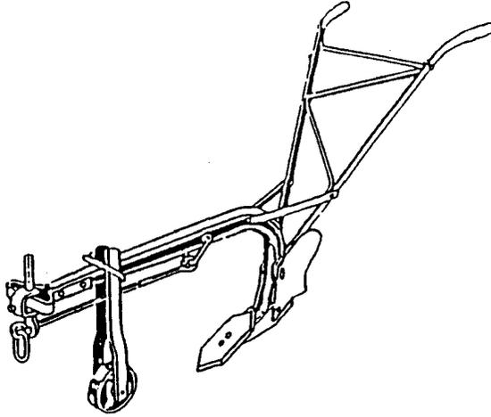
*Figure 38: Magoye ripper attachment on plough beam.*
