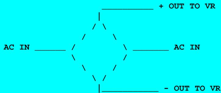
The way a bridge rectifier is wired - this is the kind in cases of two wires exiting the alternator. This may only be the first stage of an integrated rectifier/regulator unit.
