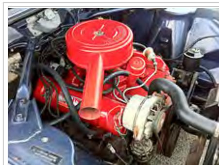
Alternator (silver) mounted on a V8 engine
