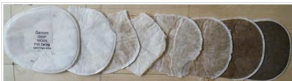
Cross-section of a disposable NIOSH P95 filter pad used in metalworking operations. Even "clean" industrial processes often generate large amounts of harmful particulate matter and require breathing protection.
